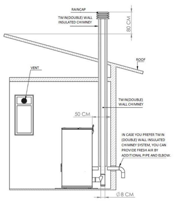
We recommend the use of twin(double) wall or twin(double) wall insulated system for chimney connection.
